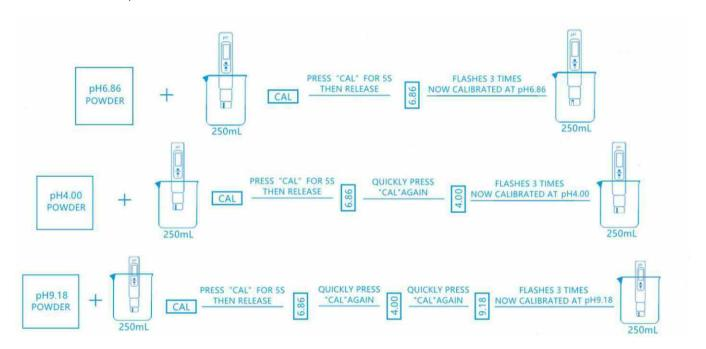
**Note:** During the calibration process, the pH pen must not leave the calibration solution. If Err (as shown in the figure below) appears, recalibration is required.
